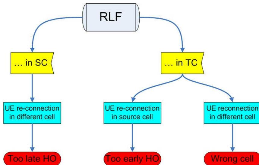
**Figure 27: Algorithms to identify the reason of a HO-failure**
