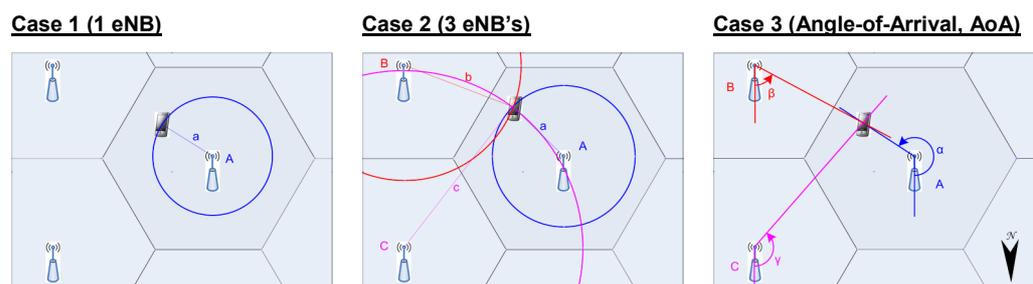
**Figure 16: Enhanced Cell ID (E-CID) methods**
