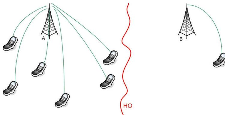
**Figure 26: Handover scenario.** The red line indicates the locations, where a handover shall be triggered.
