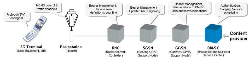
**Figure 1: MBMS network architecture for 3G networks and related tasks**
