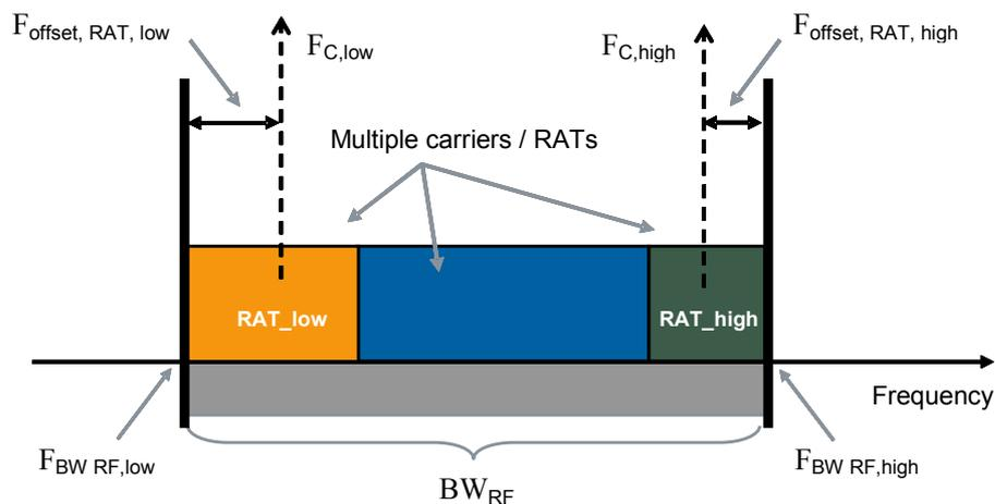
**Figure 22: Illustration of RF bandwidth related symbols and definitions for Multi-standard Radio [5]**
