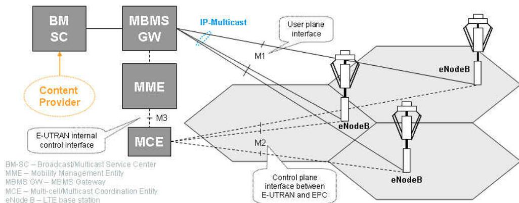
Figure 3: LTE network architecture for MBMS
