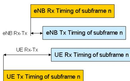
Figure 17: eNB and UE receive-transmit timing difference
