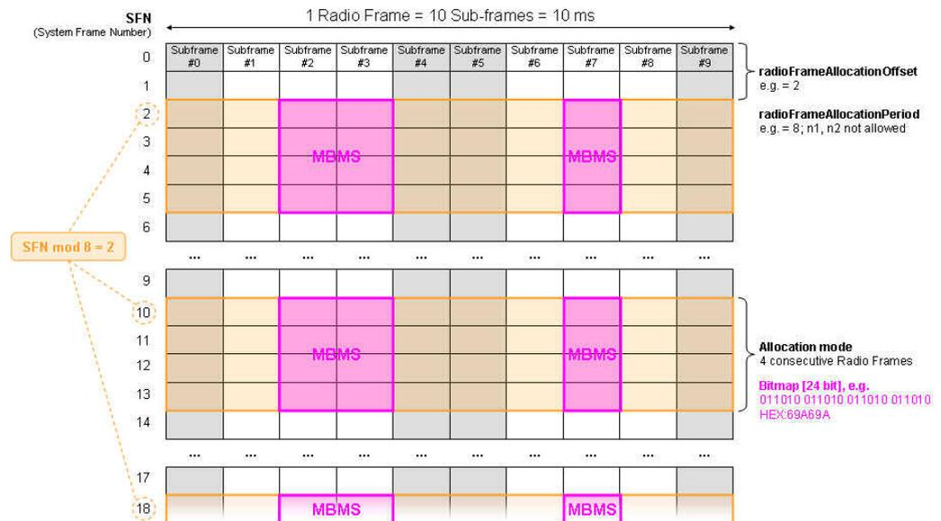
Figure 8: Determine MBSFN subframes by decoding SIB Type 2
