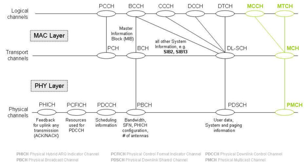
Figure 5: Enhanced channel architecture in LTE due to MBMS
