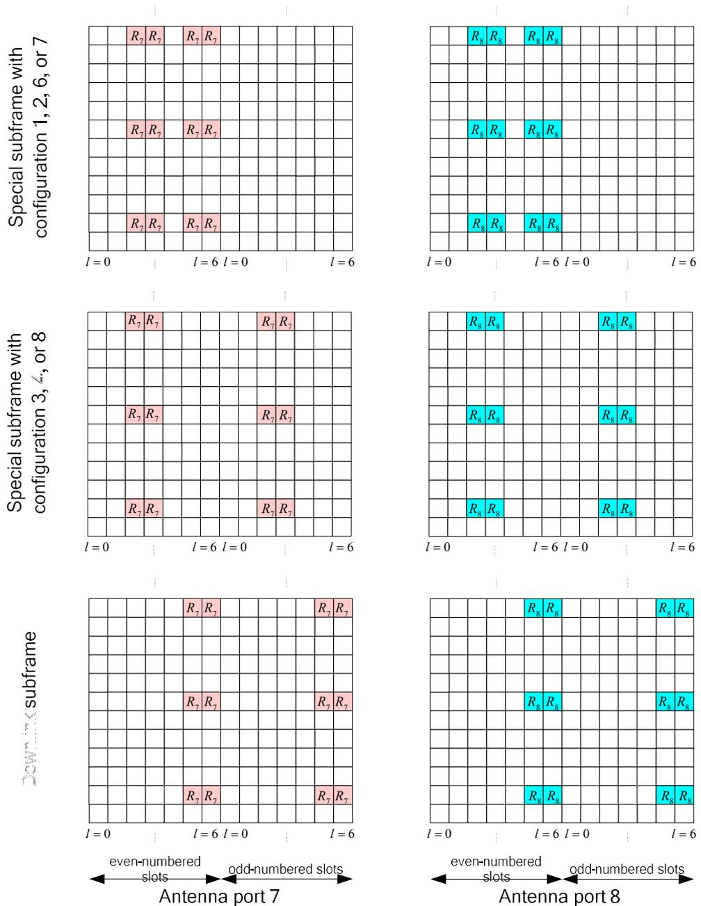
**Figure 19: Mapping of UE-specific reference signals, antenna ports 7 and 8 (normal cyclic prefix)**
