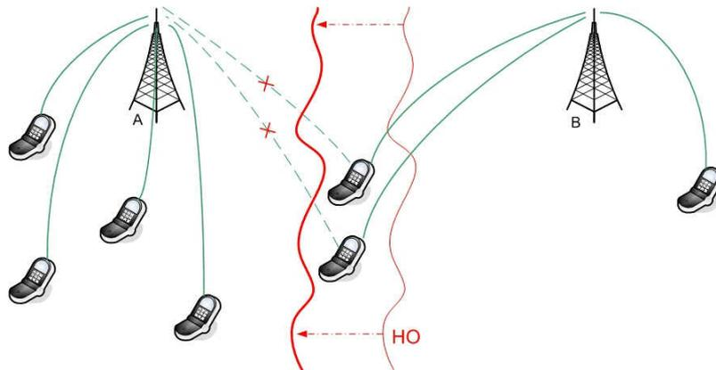
**Figure 28: Mobility Load Balancing.** The trigger line for handover is moved so that the load is better distributed between the cells.
