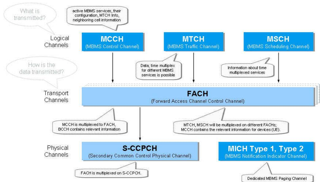
Figure 2: New 3G logical channels and physical channel due to MBMS
