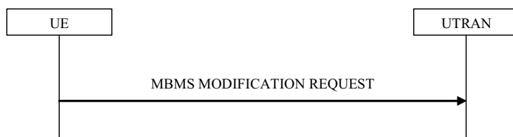
Figure 8.7.6-1: MBMS modification request, normal
