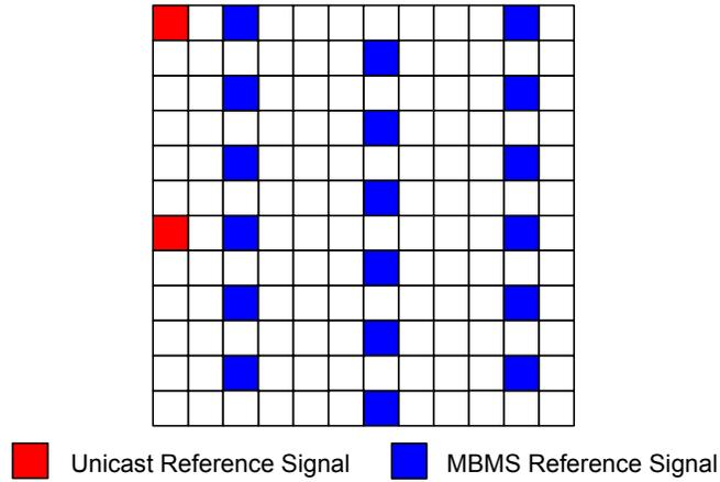
**Figure 22. Reference signal structure for mixed carrier MBSFN<sup>159</sup>**
