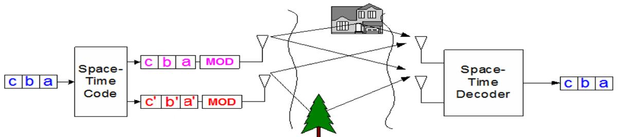
Figure 40. Illustration of Space Time Coding in a 2x2 MIMO system<sup>177</sup>
