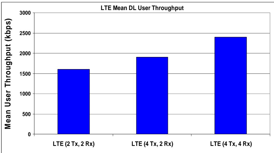
Figure 44. LTE Downlink Mean User throughput Performance with multi-antennas<sup>183</sup>
