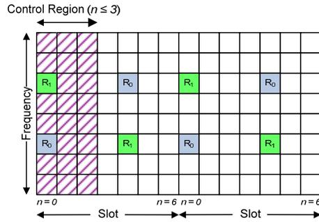
Figure 18. E-UTRA downlink sub-frame structure<sup>153</sup>
