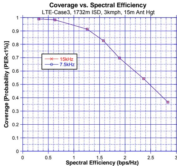
Figure 25. Coverage vs. spectral efficiency at 3km/hr<sup>161</sup>
