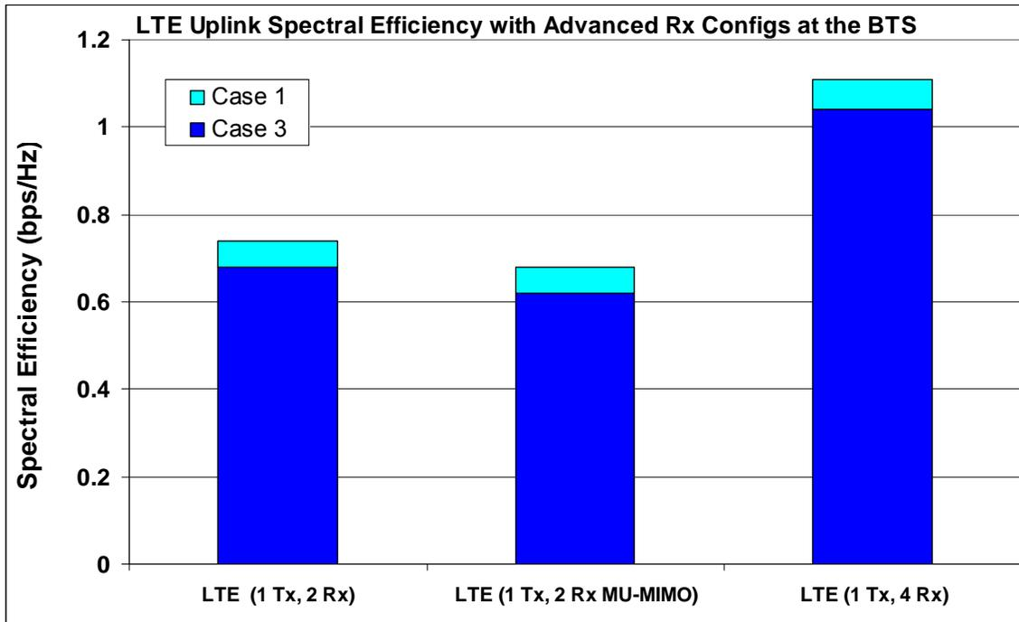
Figure 46. LTE Uplink Spectral Efficiency Performance with multi-antennas<sup>186</sup>
