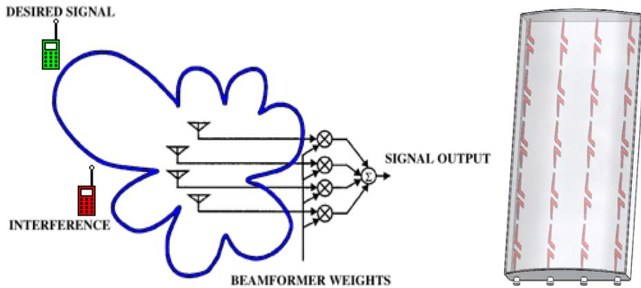
**Figure 37. Conceptual depiction of an AA system implemented with 4-column, vertically polarized planar array<sup>174</sup>**
