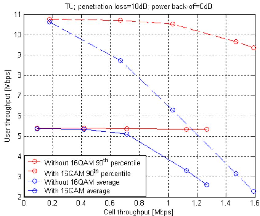
Figure 7. UL bit rate improvements with 16 QAM<sup>26</sup>
