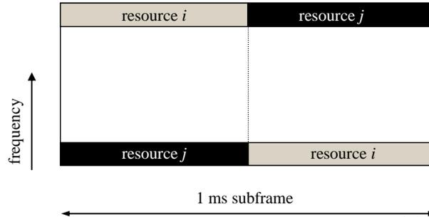
**Figure 30. Physical uplink control channel<sup>166</sup>**
