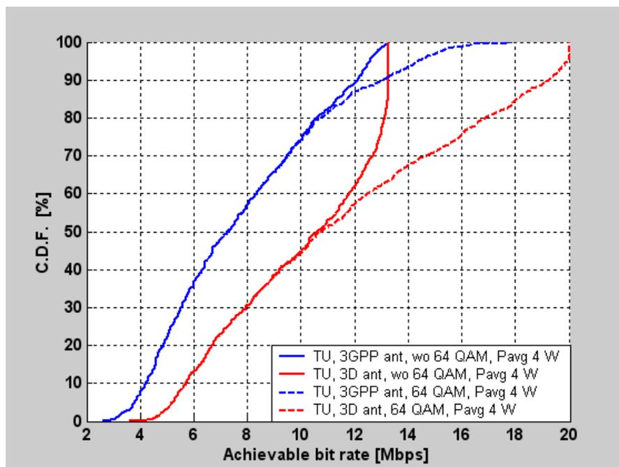
Figure 6. DL bit rate improvement with 64 QAM<sup>25</sup>
