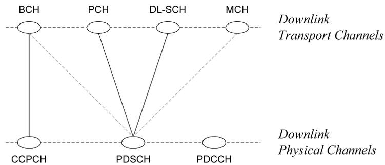
**Figure 17. Mapping between downlink transport channels and downlink physical channels<sup>151</sup>**
