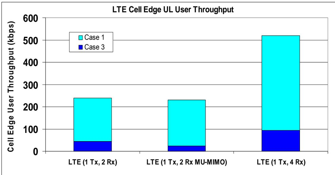
Figure 48. LTE Uplink cell edge performance with multi-antennas<sup>188</sup>
