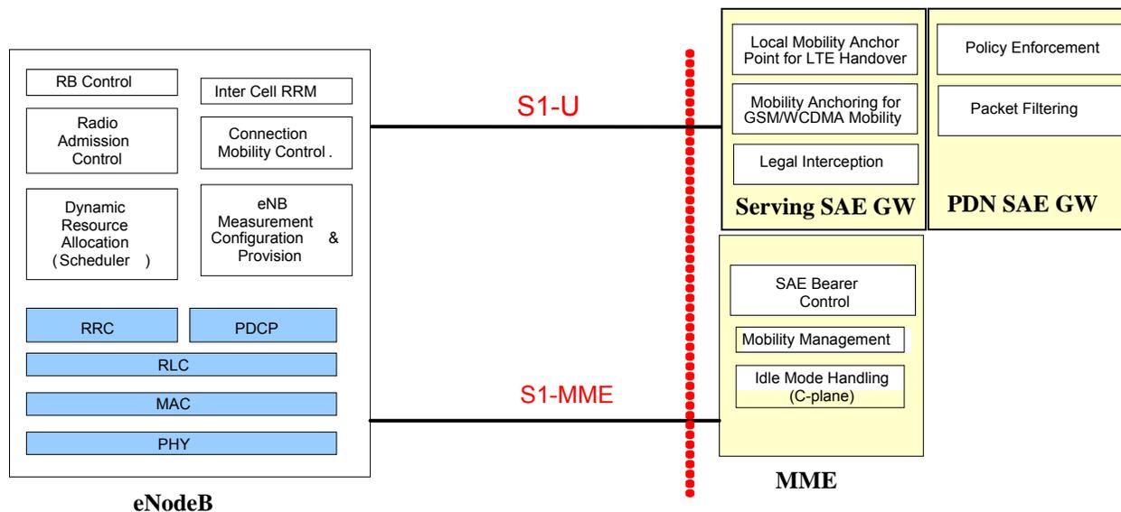
**Figure 36. Functional Split between radio access and core network**<sup>173</sup>
