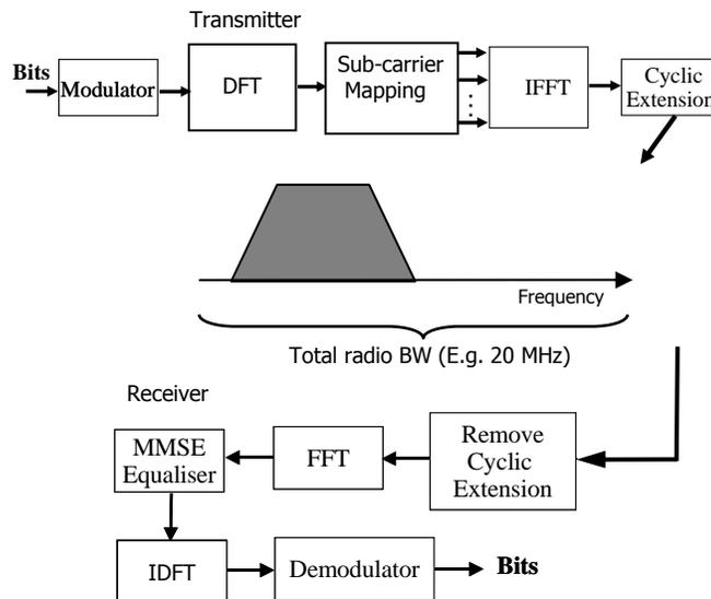
**Figure 27. SC-FDMA transmitter and receiver chains with frequency domain equalization<sup>163</sup>**
