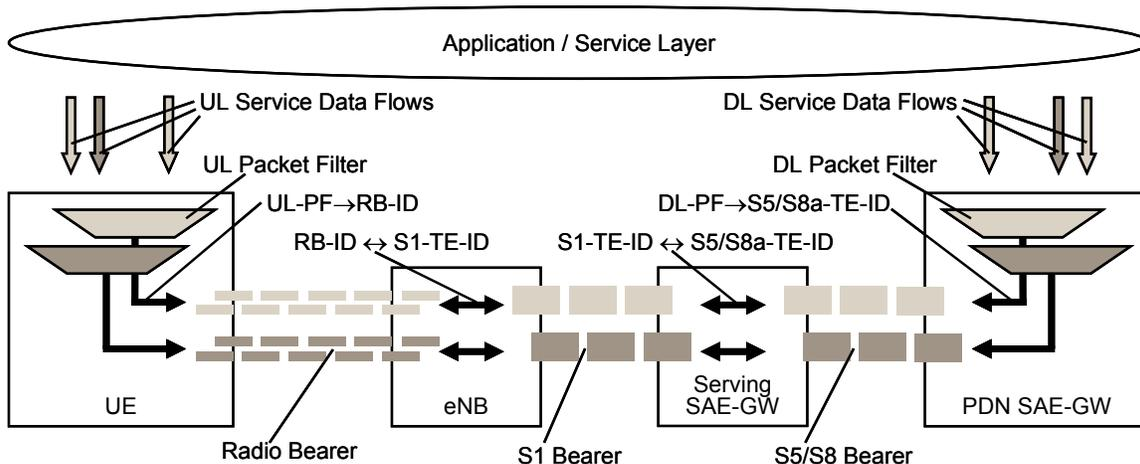
**Figure 11. Two Unicast bearers (GTP-u Based S5/S8)<sup>145</sup>**
