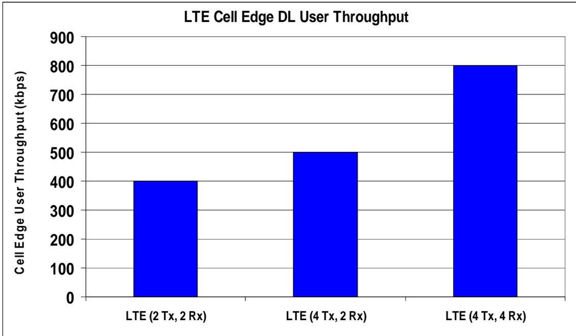
Figure 45. LTE Downlink Cell EDGE Performance with multi-antennas<sup>184</sup>
