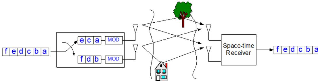
**Figure 41. Illustration of Spatial Multiplexing in a 2x2 MIMO system<sup>178</sup>**
