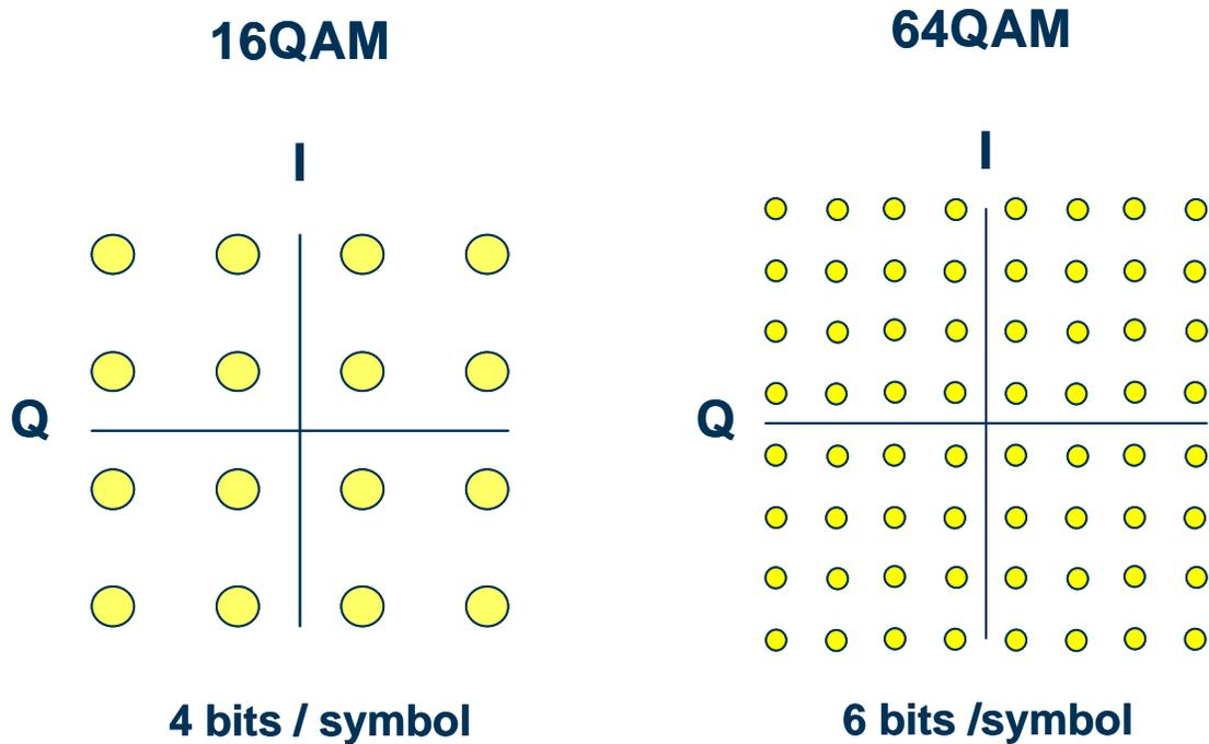
**Figure 3. Typical 16QAM and 64QAM Constellations<sup>17</sup>**
