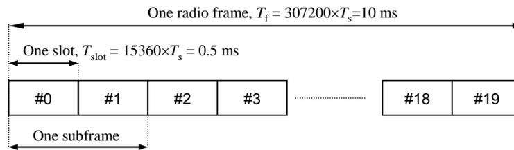
**Figure 29. Frame structure type 1<sup>165</sup>**
