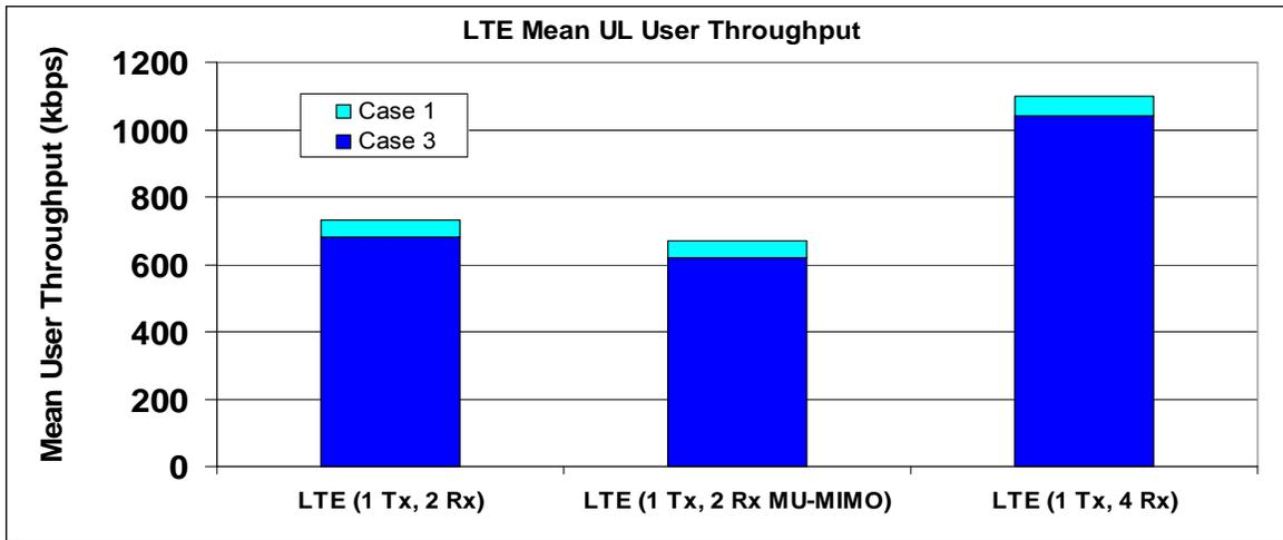
Figure 47. LTE Uplink Mean Throughput Performance with multi-antennas<sup>187</sup>
