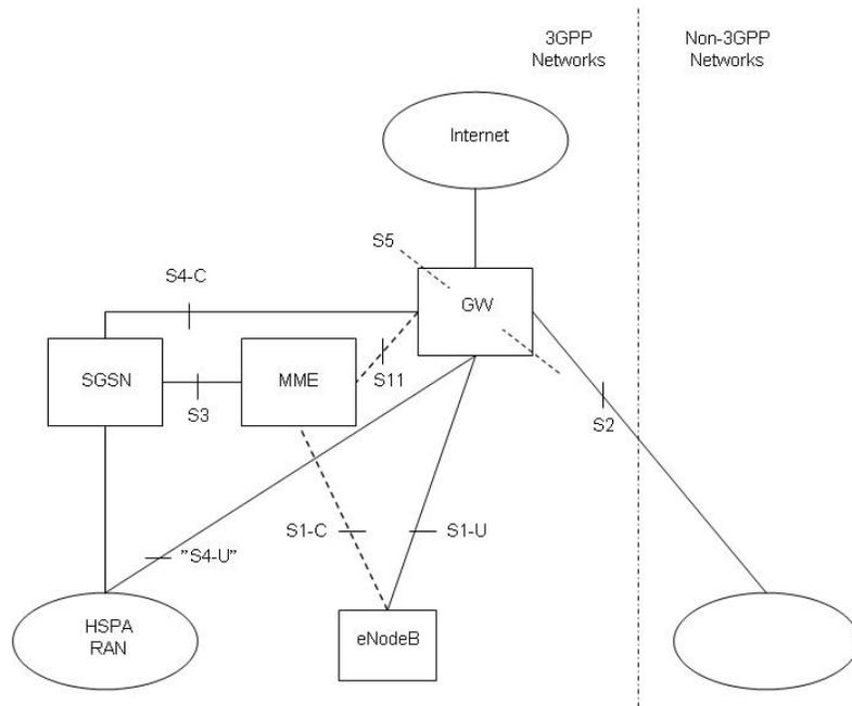
**Figure 9. Example configuration for EPS support of Rel-7 UMTS/HSPA and non-3GPP accesses<sup>143</sup>**
