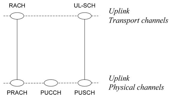
**Figure 28. Mapping between uplink transport channels and uplink physical channels<sup>164</sup>**
