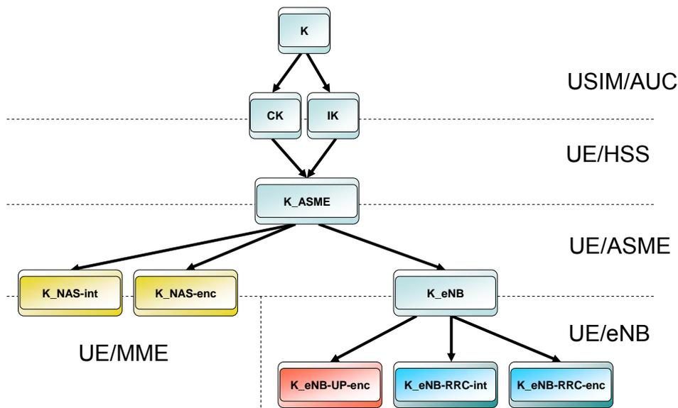
*Note: An Access Security Management Entity (ASME) is a new functional entity which receives the top-level keys in an access network from the HSS, i.e., the MME.*
