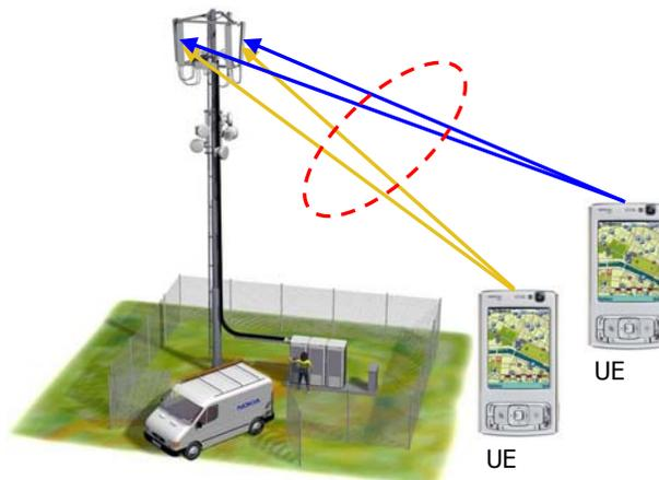
**Figure 42. The basic principle of uplink MU-MIMO with 2x2 antenna configuration<sup>179</sup>**
