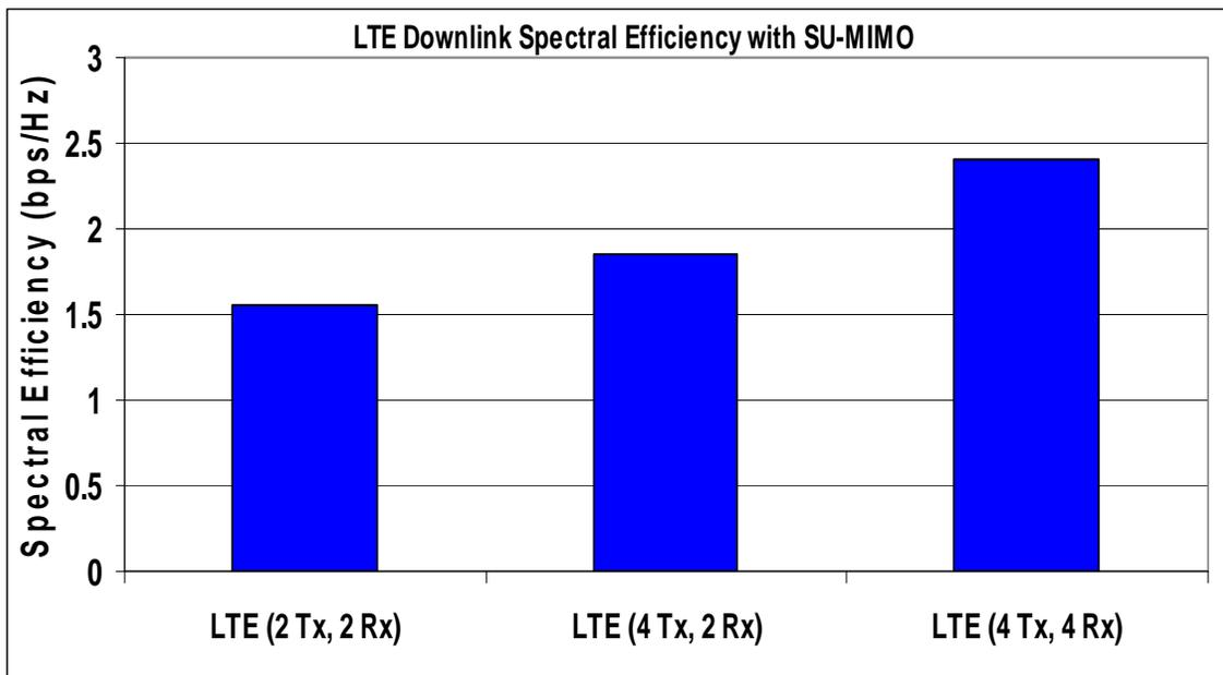
Figure 43. LTE Downlink Spectral Efficiency Performance with multi-antennas<sup>182</sup>
