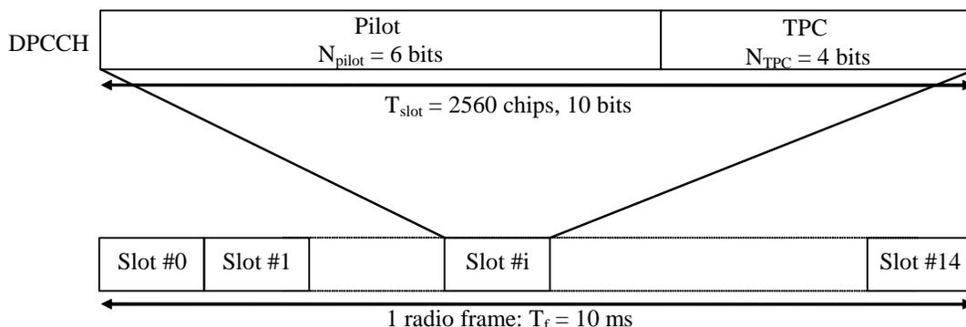
**Figure 4. New DPCCH slot format<sup>20</sup>**
