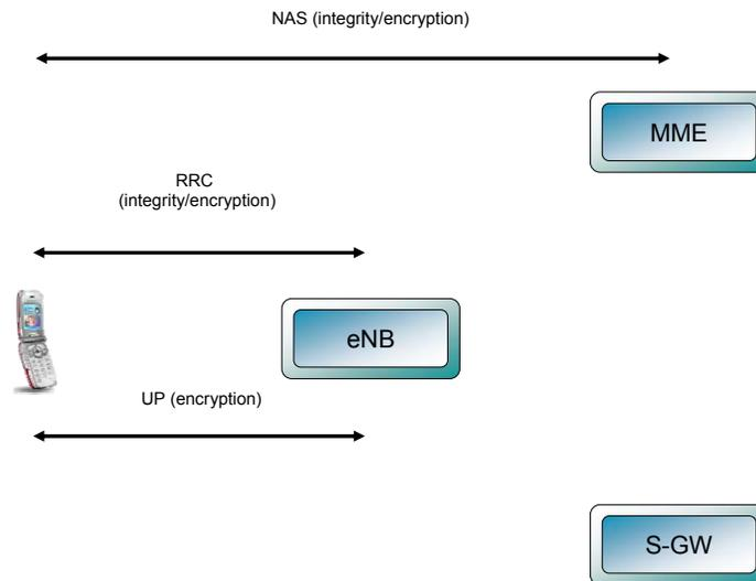
**Figure 13. Security termination points for traffic to/from the UE<sup>147</sup>**
