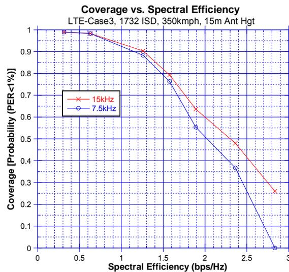
**Figure 26. Coverage vs. spectral efficiency at 350kmph<sup>162</sup>**
