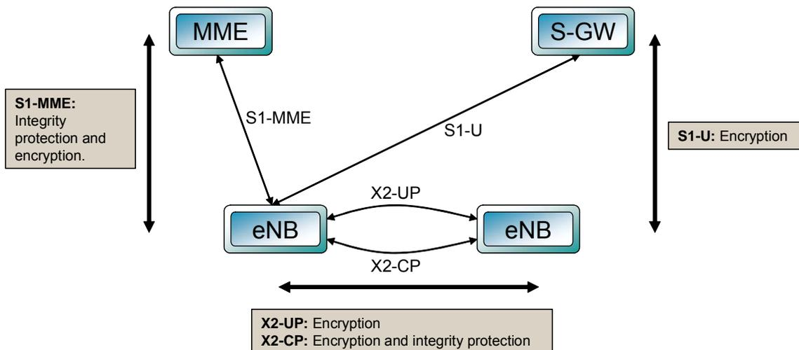
**Figure 14. Security termination points for traffic internal to EPS<sup>148</sup>**
