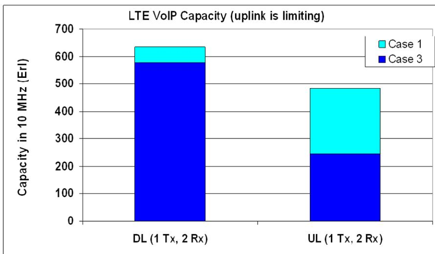
Figure 34. LTE VoIP capacity<sup>171</sup>
