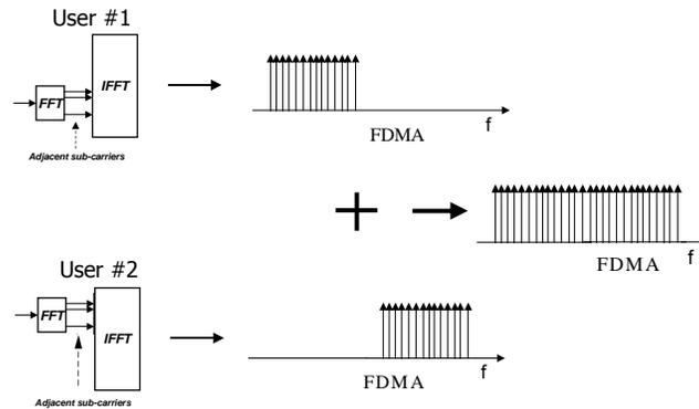
**Figure 35. The principle of frequency domain scheduling in EUTRAN<sup>172</sup>**
