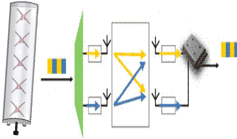
Figure 39. Conceptual depiction of a 2x2 MIMO system implemented with dual-pole, slant-45 base station antenna and two antennas in the UE<sup>176</sup>
