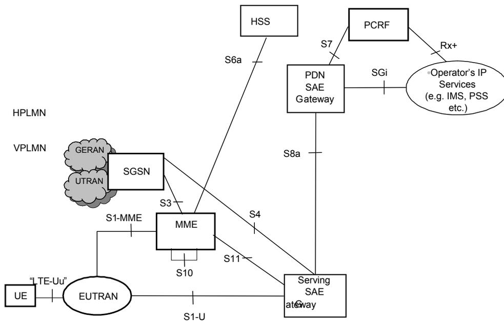
Figure 5. Roaming architecture (home routed case, 3GPP only networks)<sup>149</sup>
