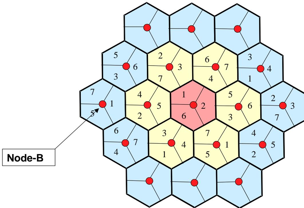
**Figure 49. Cell planning for inverted re-use 7 scheme (FFR=6/7)<sup>189</sup>**
